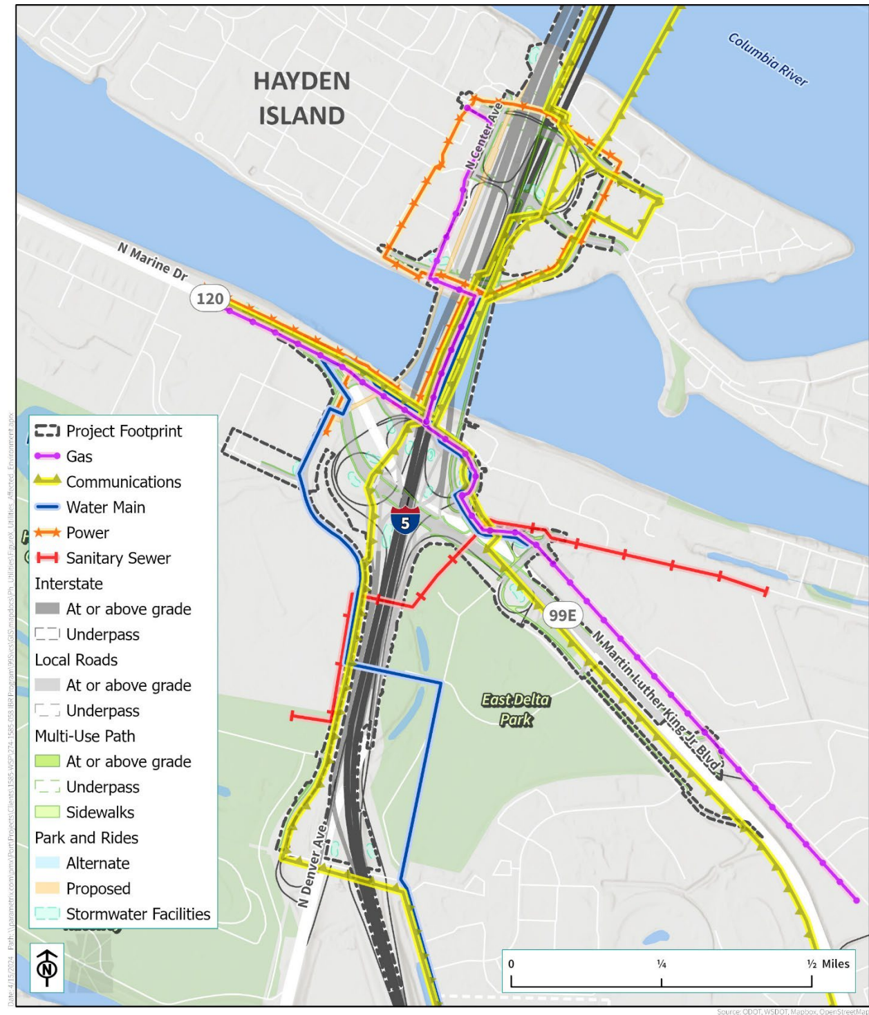
Figure 4-1. Impacts to Existing Major Utilities in Oregon Study Area
