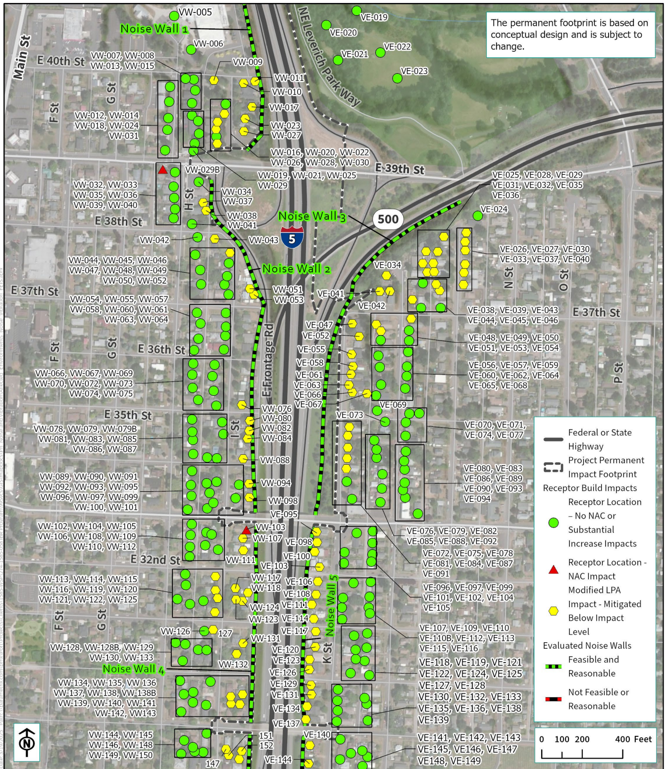
Figure 3.11-20. Modified LPA with Recommended Design Options – 2045 Evaluated Noise Walls – E 30th Street to E 39th Street
