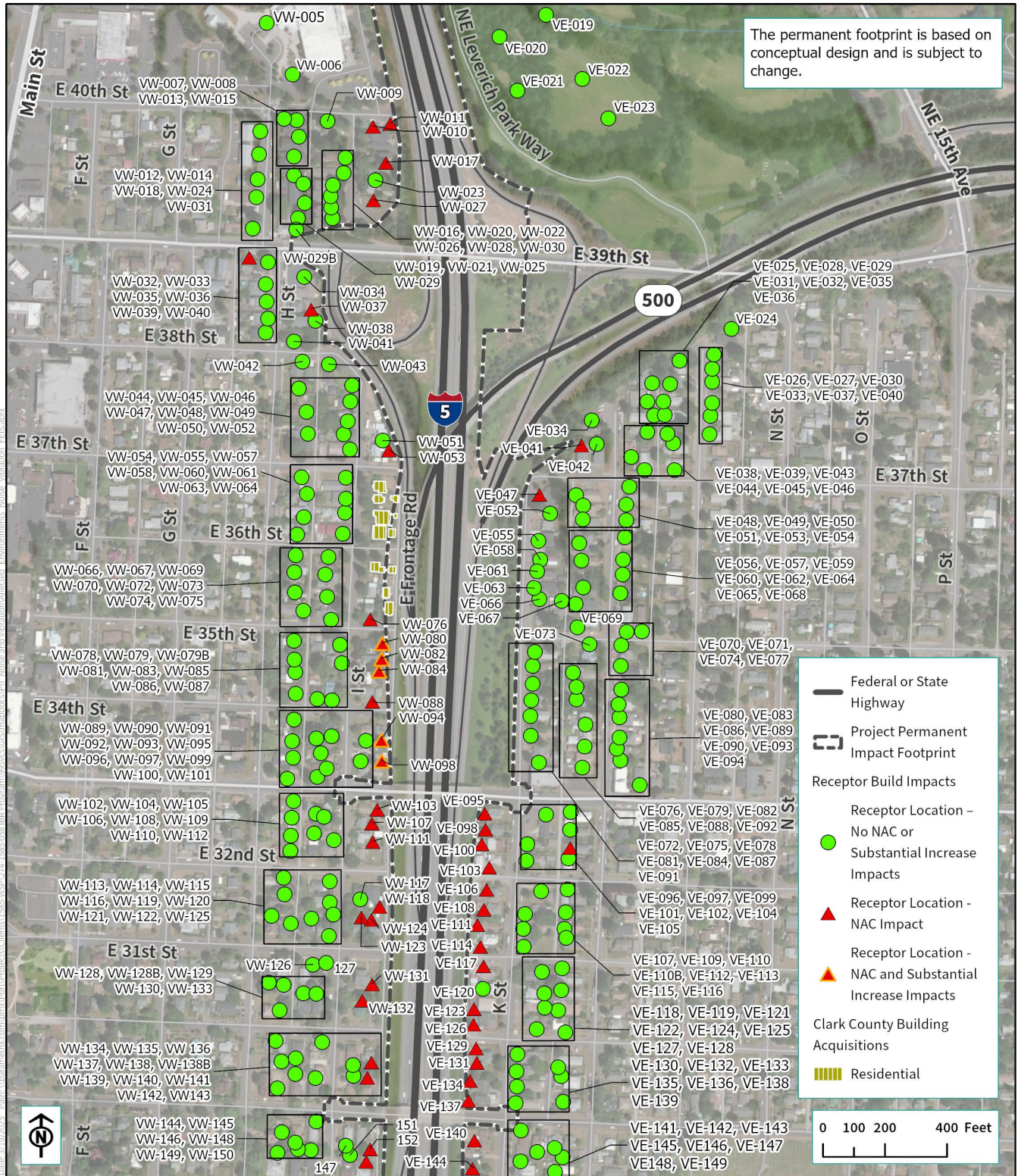
Figure 3.11-11. Modified LPA with Recommended Design Options – 2045 Traffic Noise Impacts – E 30th Street to E 39th Street
