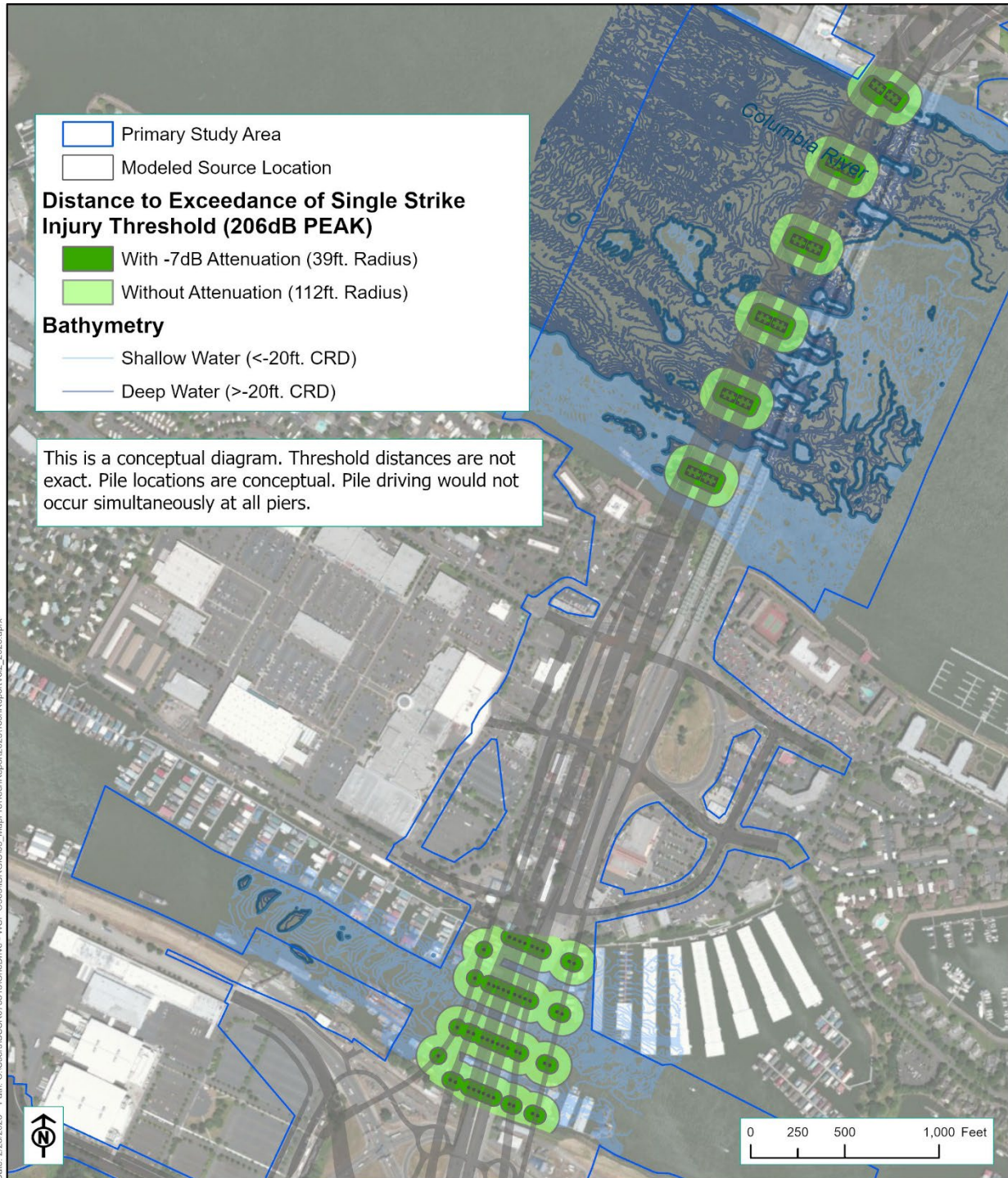
Figure 5-4. Distance to 206 dB Peak Injury Threshold for Fish During Impact Pile Driving – 36- to 48-inch Pile
