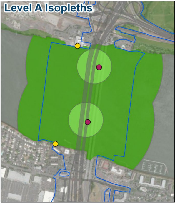
Figure 5-16. Level A and B Underwater Isopleths During Impact Pile Driving - Two Pile Drivers; With Bubble Curtain
