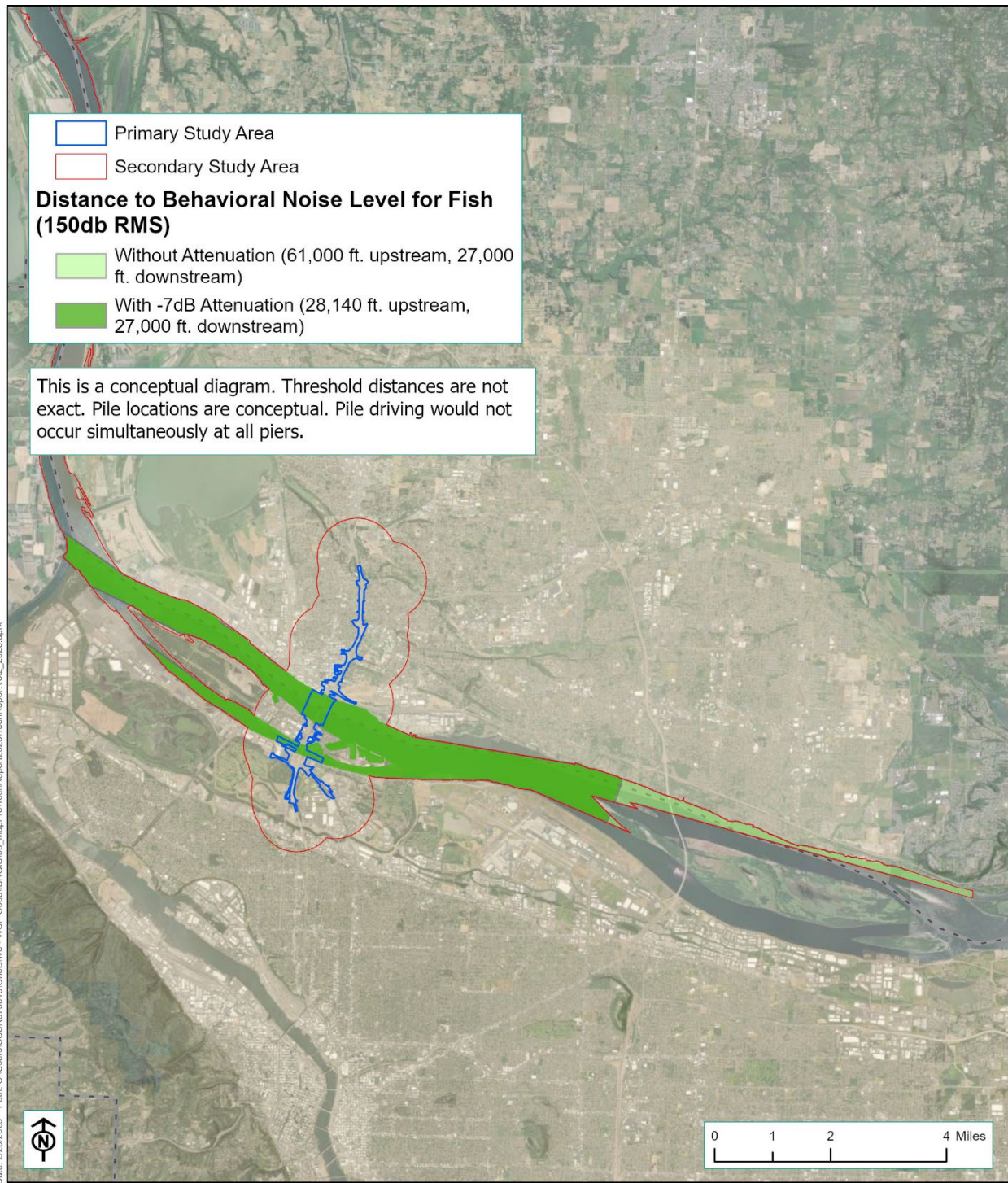
Figure 5-12. Distance to 150 dB RMS Disturbance Thresholds during Impact Pile Driving – 36- to 48-inch Pile
