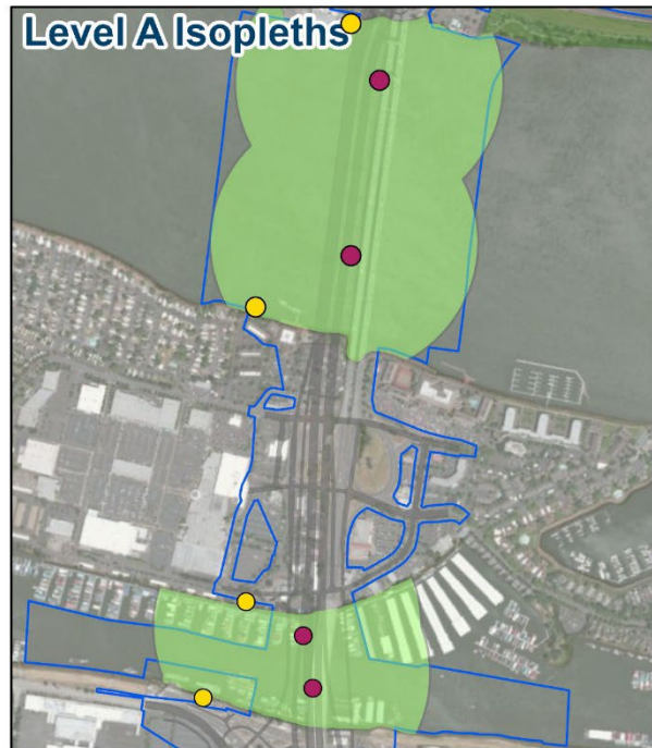
Figure 5-18. Level A and B Underwater Isoleths During Vibratory Pile Driving - Two Pile Drivers
