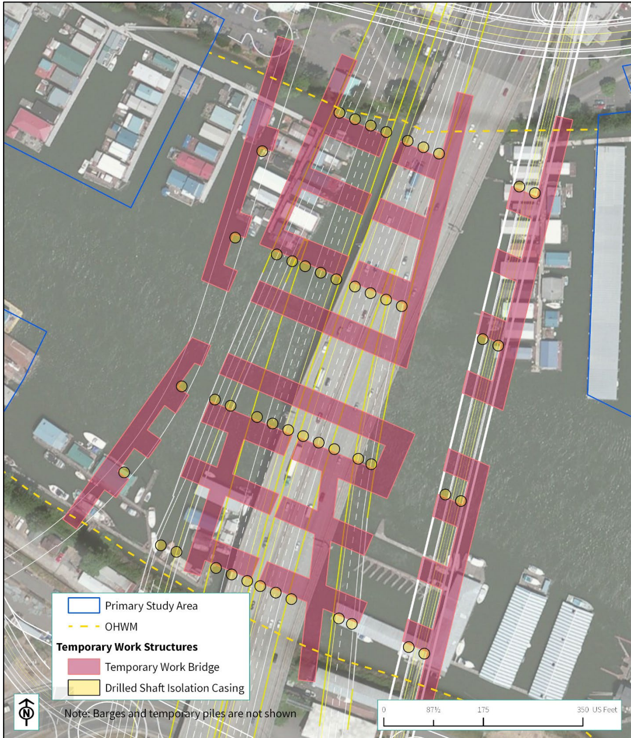
Figure 5-2. Temporary Work Structures – North Portland Harbor
