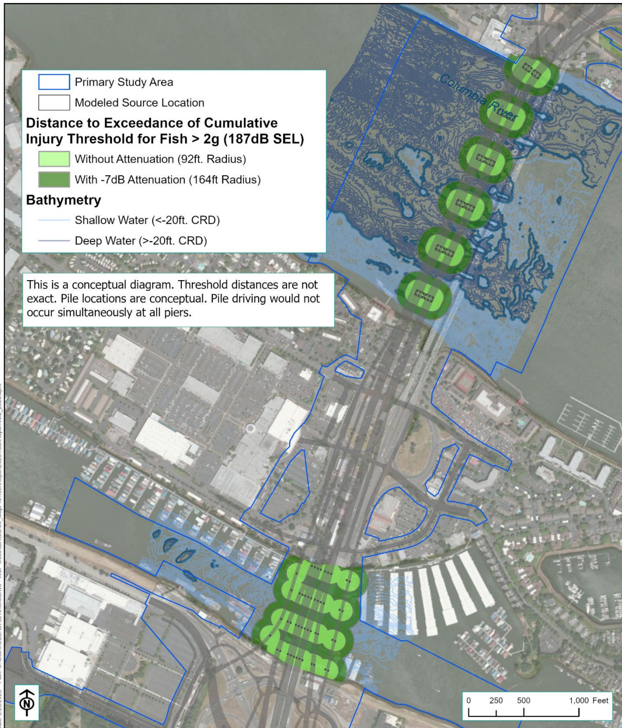
Figure 5-7. Distance to 187 dB SEL Cumulative Injury Threshold for Fish >2 g during Impact Pile Driving – 18- to 24-inch Pile, Single Pile Driver
