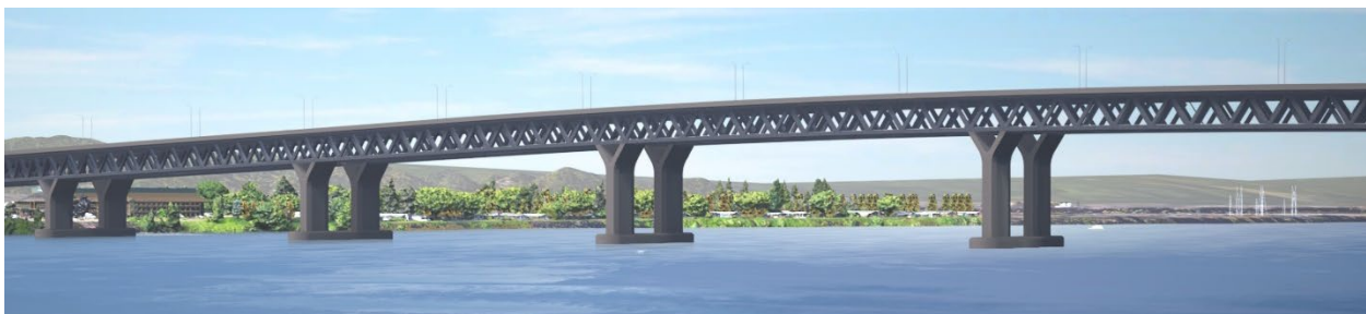
Figure 1-19. Conceptual Drawing of a Double-Deck Fixed-Span Configuration
