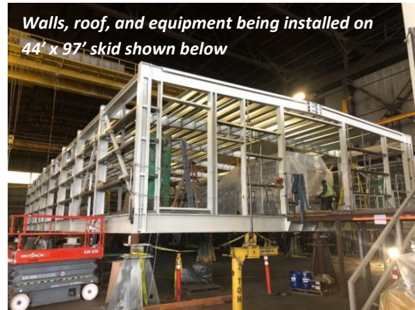
Shown below in late 2019, this skid represents the largest non-oil related module manufactured by TMF. At 44' W x 97' L, this module is too large to ship over the road, and too big to be handled in the field.
