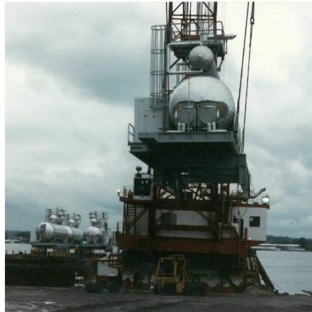
Process vessels and skids are being loaded on a barge from Thompson Metal Fab's facility. This load will be delivered to Alaska and used on the North Slope. These units are well over 20' and 40' long.
