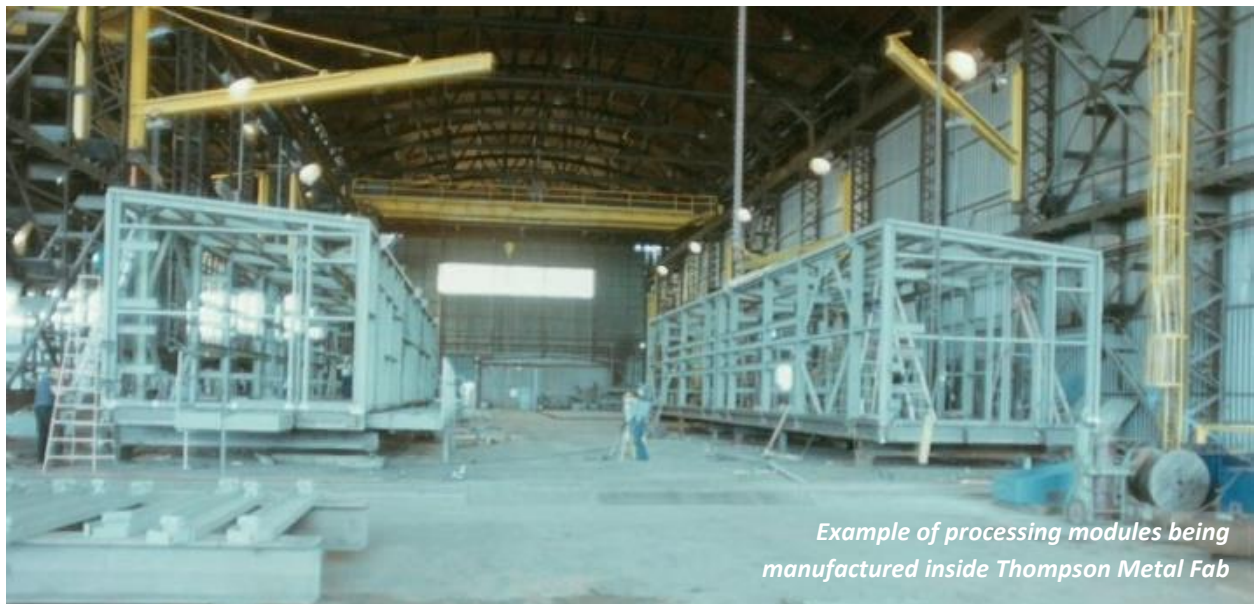
Enclosed modules to be used for a drilling rig, shown inside TMF’s shop
