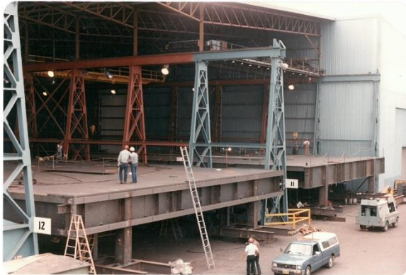
Massive platforms for the Alaska oilfields being fabricated at Thompson Metal Fab in the mid-1980's. The platforms nearly took up the entire width of a bay (80')
