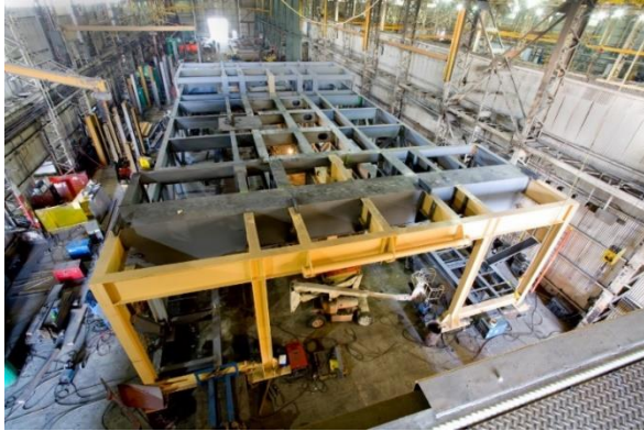
Shown above is the part of the substructure base for Rig 272. Its twin (Rig 273) was manufactured at the same time at TMF. Picture below shows the yard assembly of Rig 272, Rig 273, and Rig 25.
