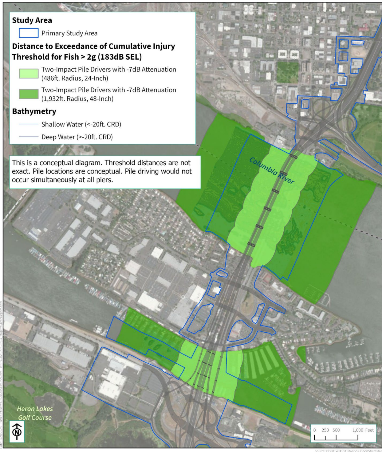
Figure 5-11. Distance to 183 dB SEL Cumulative Injury Threshold for Fish <2 g during Impact Pile Driving – All Pile Sizes, Multiple Pile Drivers
