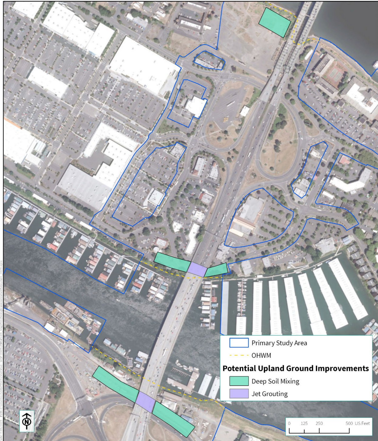
Figure 5-3. Potential Upland Ground Improvements
