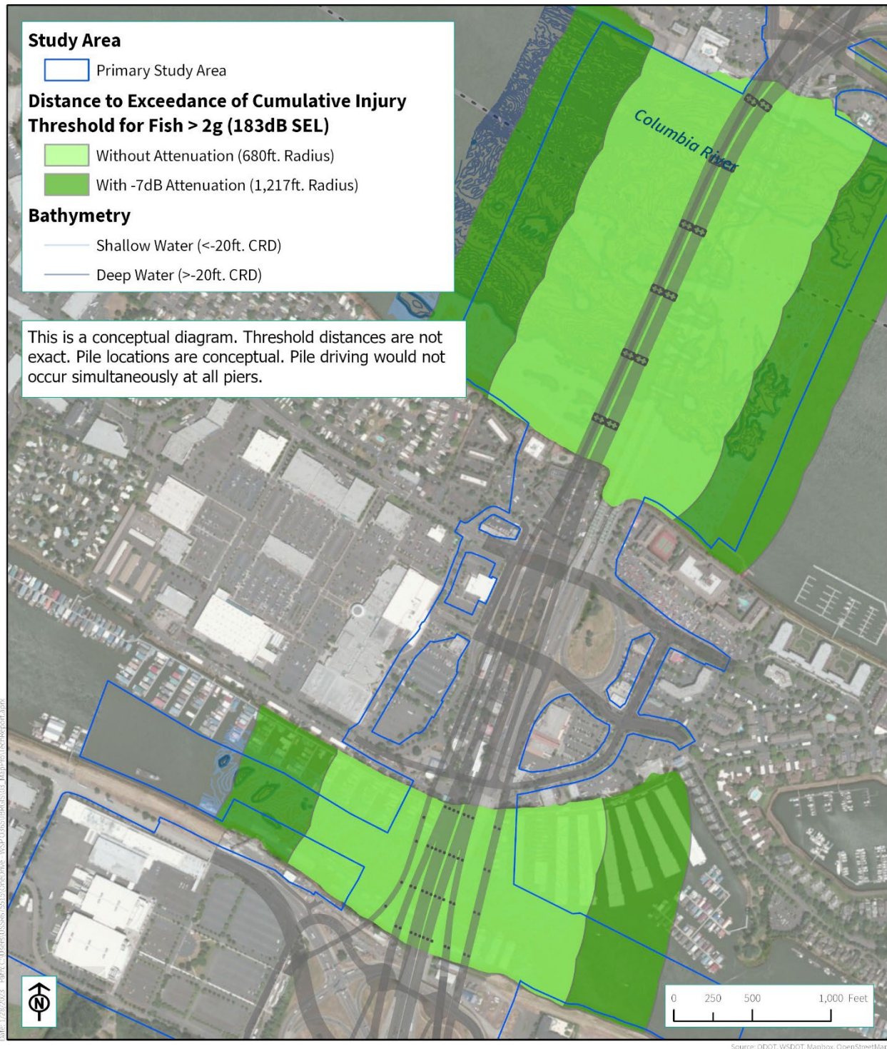
Figure 5-9. Distance to 183 dB SEL Cumulative Injury Threshold for Fish <2 g During Impact Pile Driving – 36- to 48-inch Pile, Single Pile Driver
