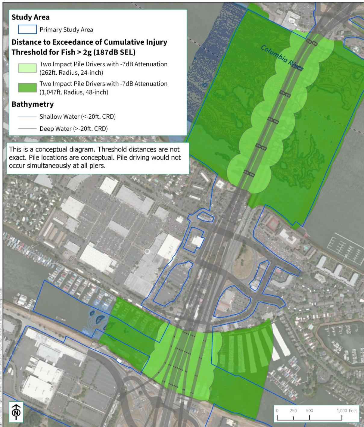
Figure 5-8. Distance to 187 dB SEL Cumulative Injury Threshold for Fish >2 g during Impact Pile Driving – All Pile Sizes, Multiple Pile Drivers
