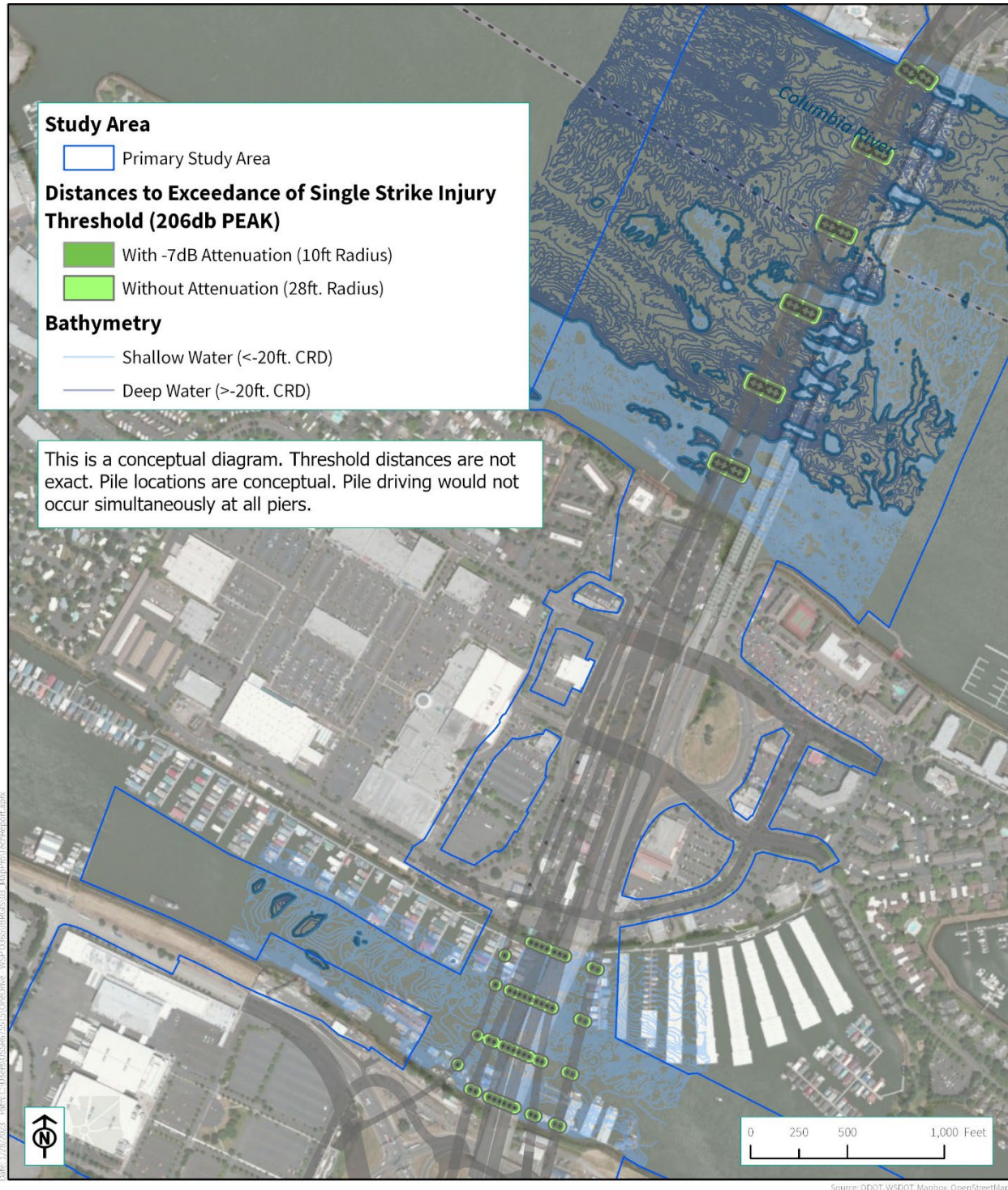
Figure 5-5. Distance to 206 dB Peak Injury Threshold for Fish during Impact Pile Driving – 18- to 24-inch Pile
