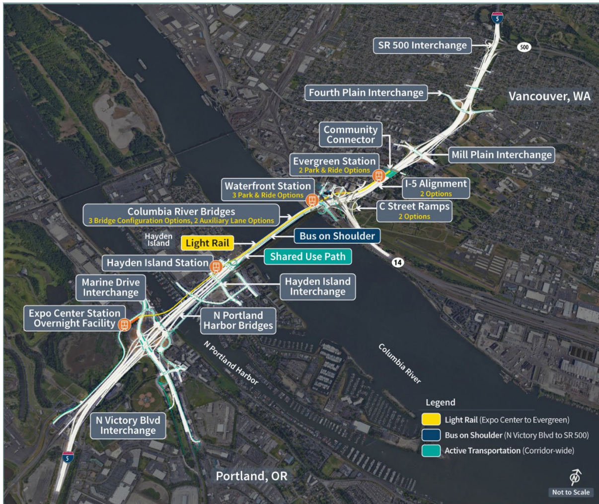
Figure 1-2. Modified LPA Components
