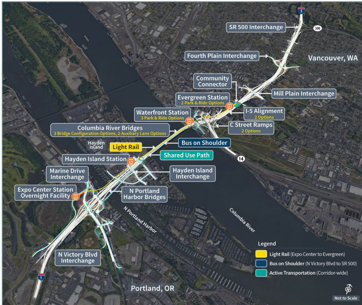
Figure 1-2. Modified LPA Components
