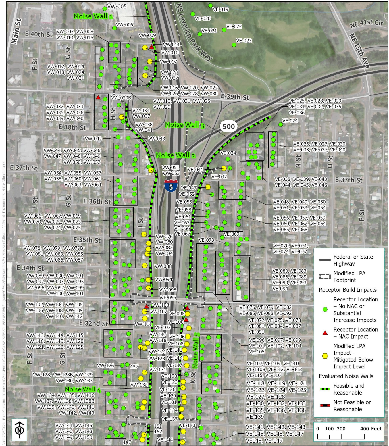
Figure 3.11-19. Modified LPA with Double-Deck Bridge Fixed-Span Configuration and One Auxiliary Lane – 2045 Evaluated Noise Walls – E 30th Street to E 39th Street
