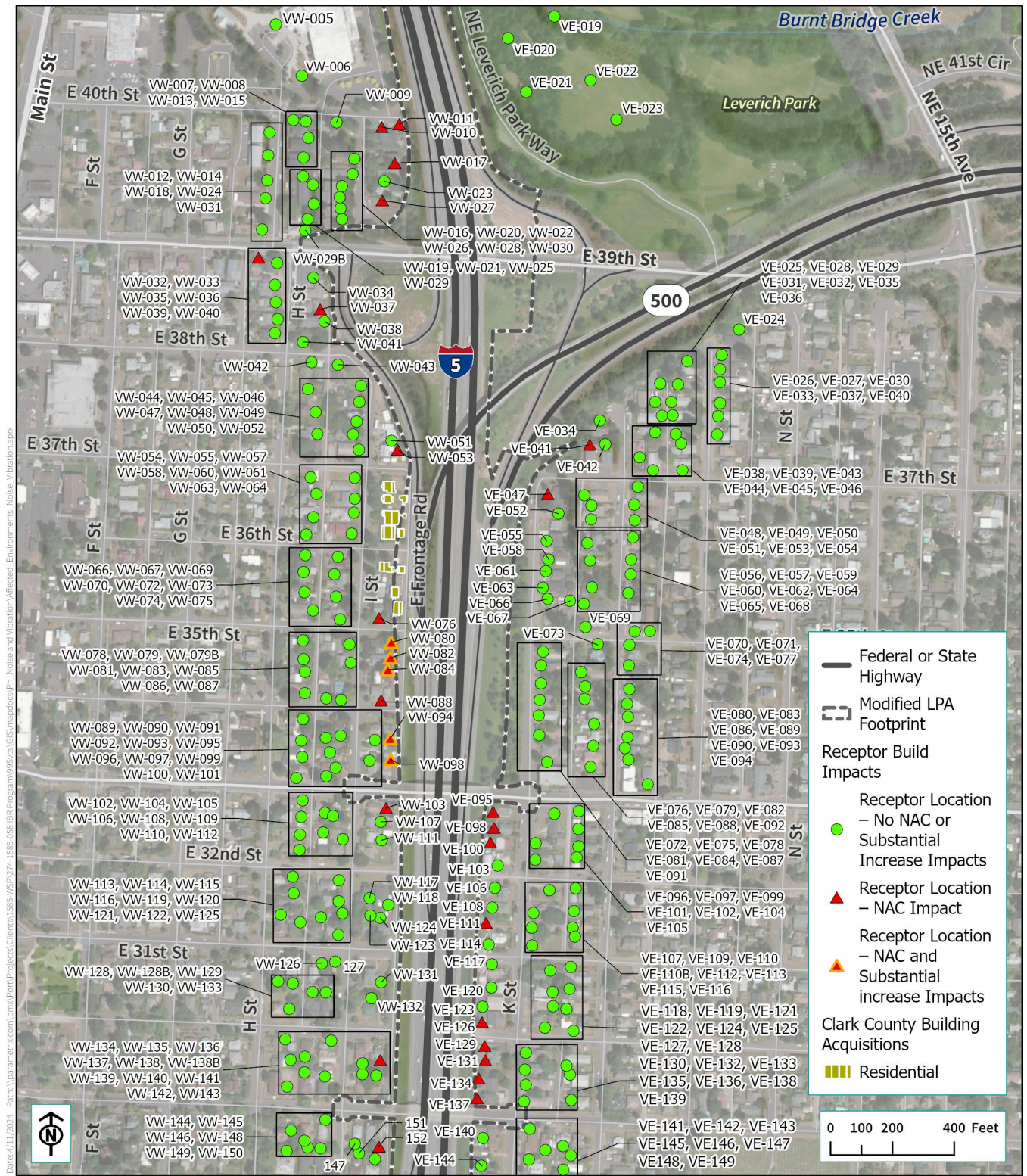
Figure 3.11-10. Modified LPA with Double-Deck Fixed-Span Configuration and One Auxiliary Lane – 2045 Traffic Noise Impacts – E 30th Street to E 39th Street
