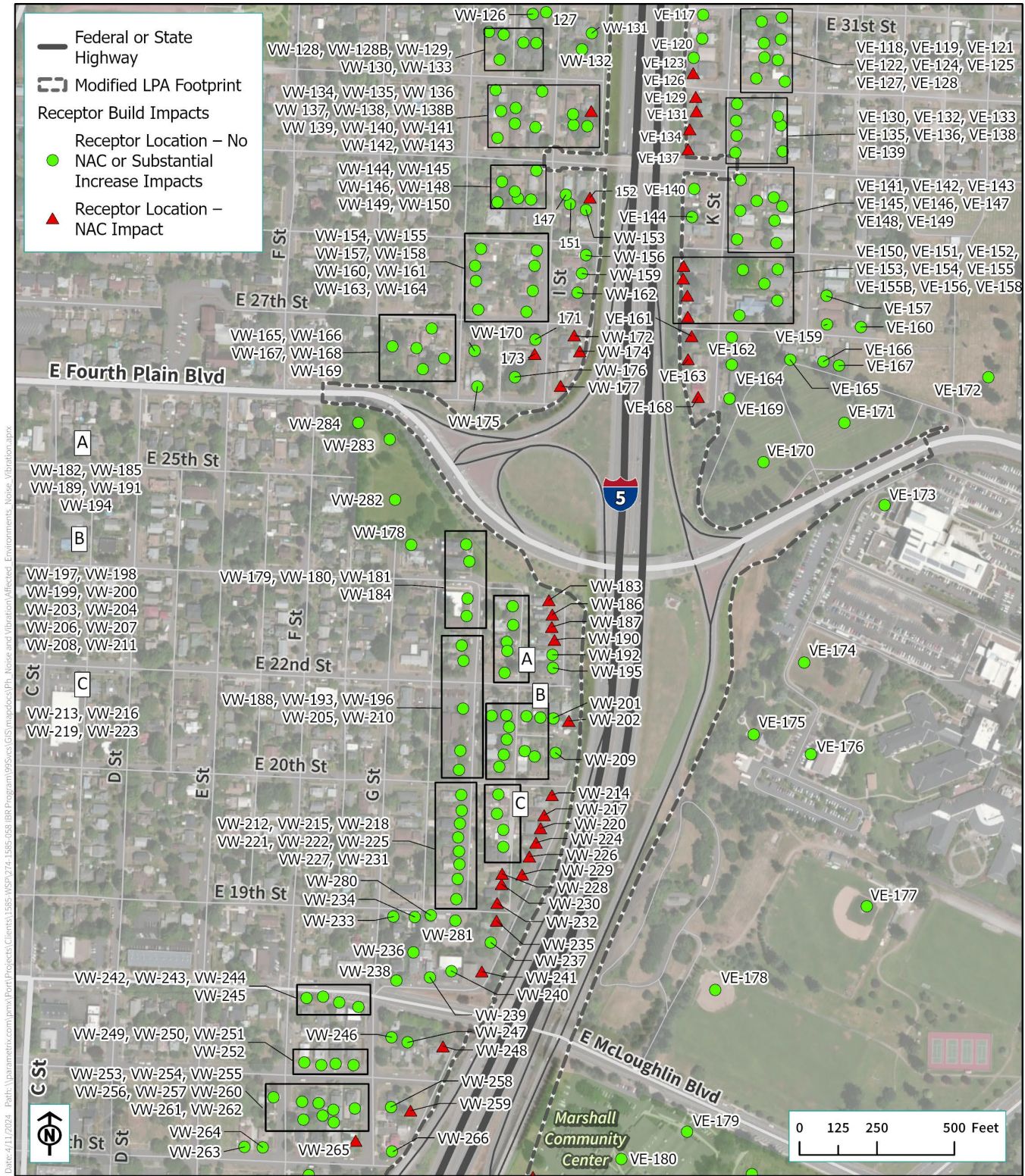
Figure 3.11-9. Modified LPA with Double-Deck Fixed-Span Configuration and One Auxiliary Lane – 2045 Traffic Noise Impacts – McLoughlin Boulevard to E 30th Street
