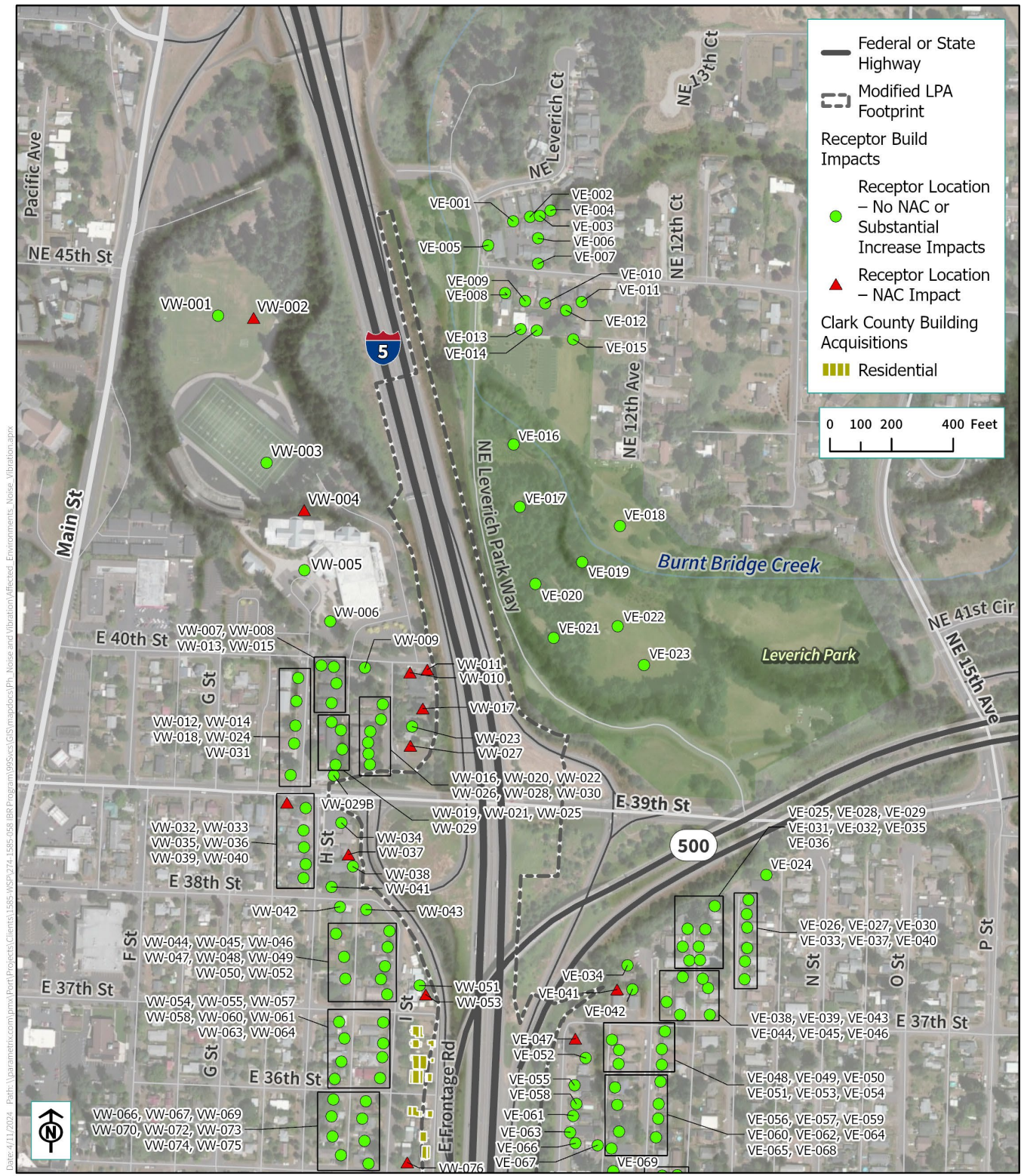
Figure 3.11-11. Modified LPA with Double-Deck Fixed-Span Configuration and One Auxiliary Lane – 2045 Traffic Noise Impacts – E 39th Street to Terminus
