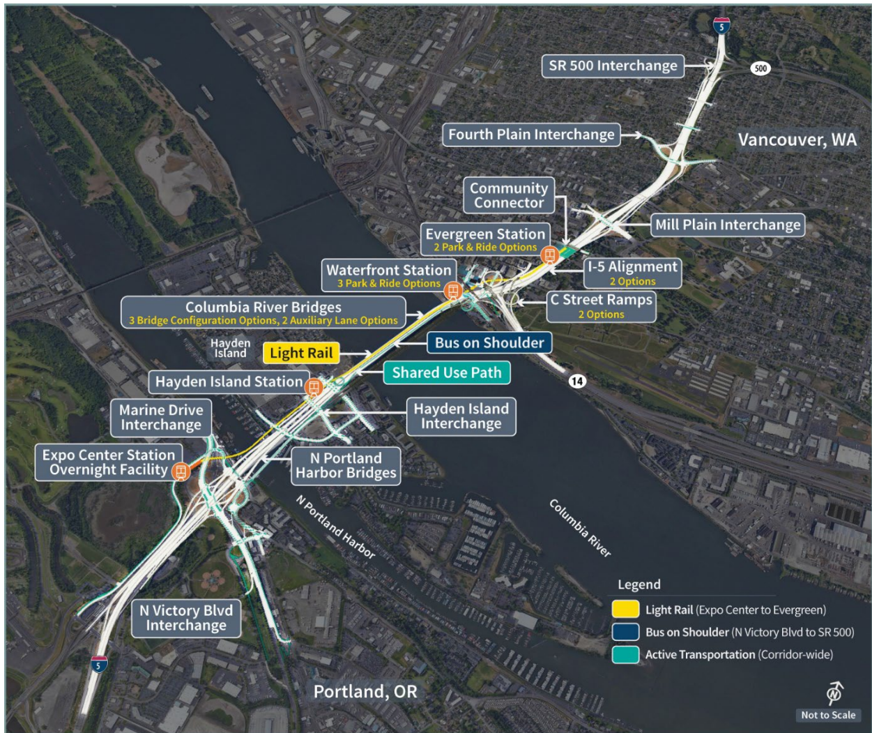
Figure 1-2. Modified LPA Components
