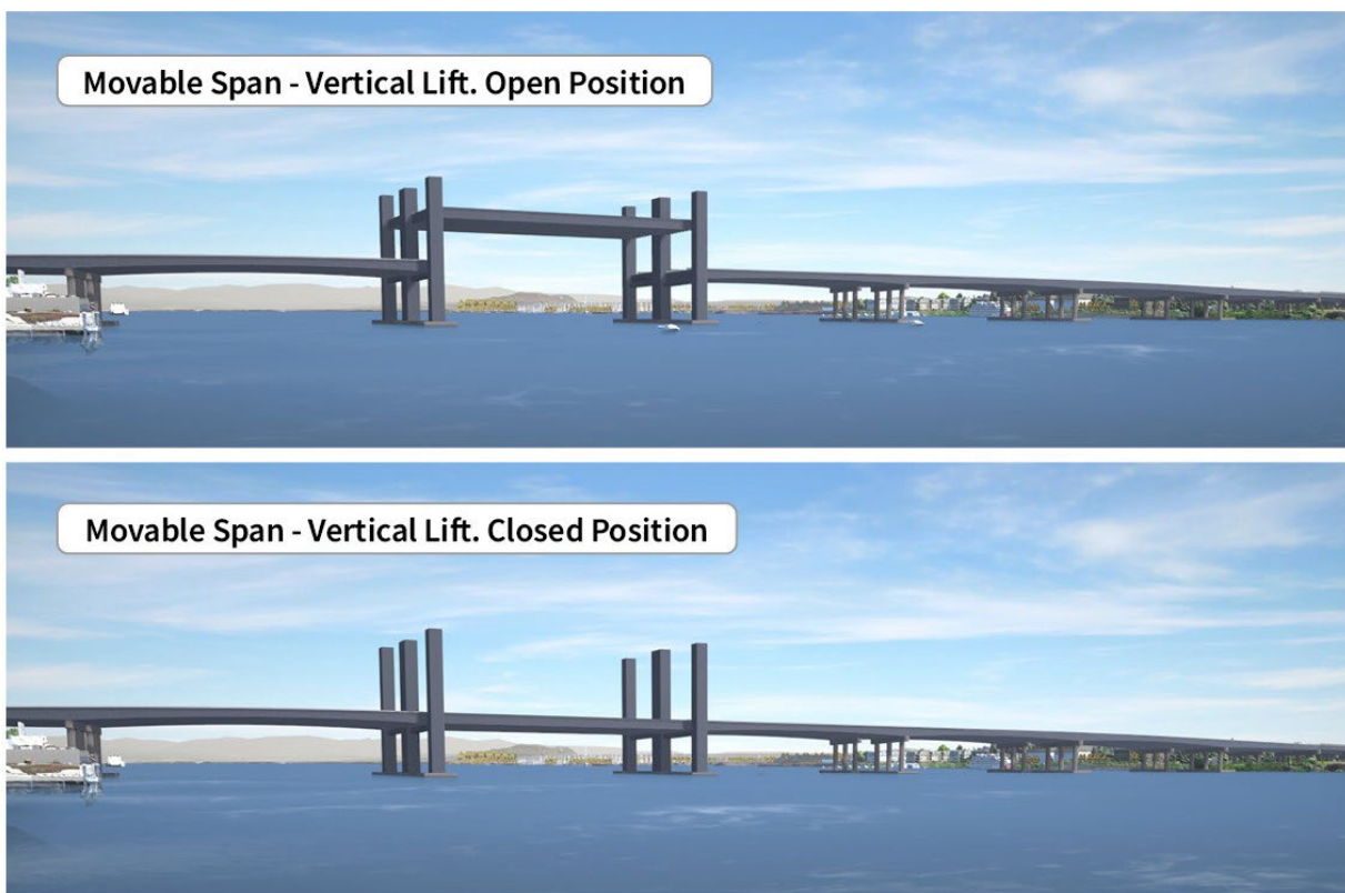
Figure 1-19. Conceptual Drawings of Single-Level Movable-Span Configurations in the Closed and Open Positions
